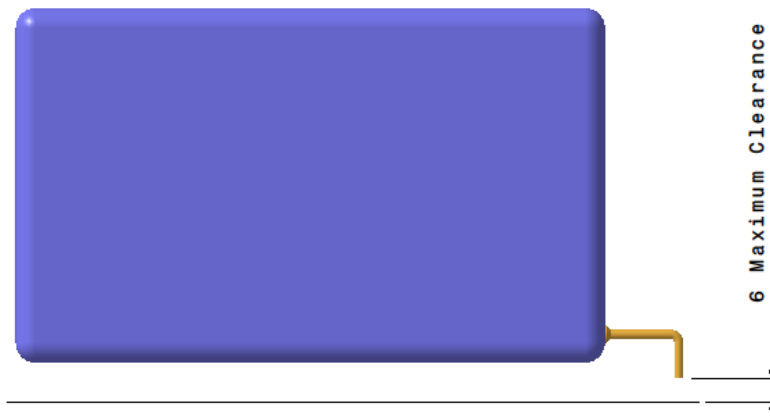
Figure 7: The Datum Pointer must be no more than 6mm above the lane surface.
