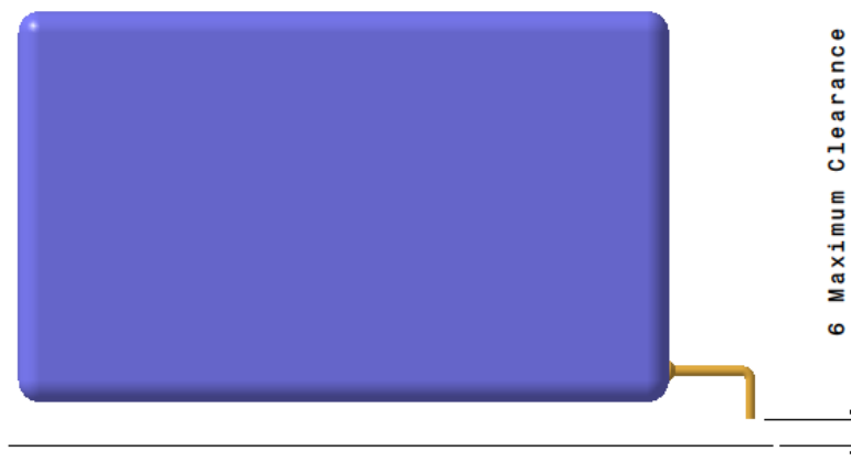
Figure 9: The Datum Pointer must be no more than 6mm above the lane surface.
